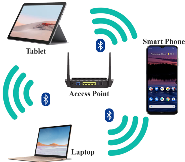
Figure 2.12 Bluetooth PAN configuration
