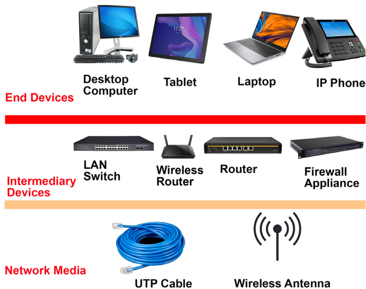
Figure 2.2 End devices, intermediary devices and media
