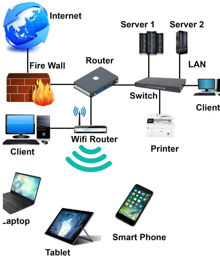
Figure 2.13 Wired and wireless and local area networks
